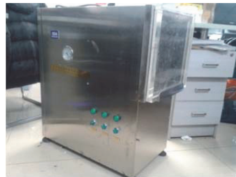
FIGURE 14: Vacuum deaeration tank.
